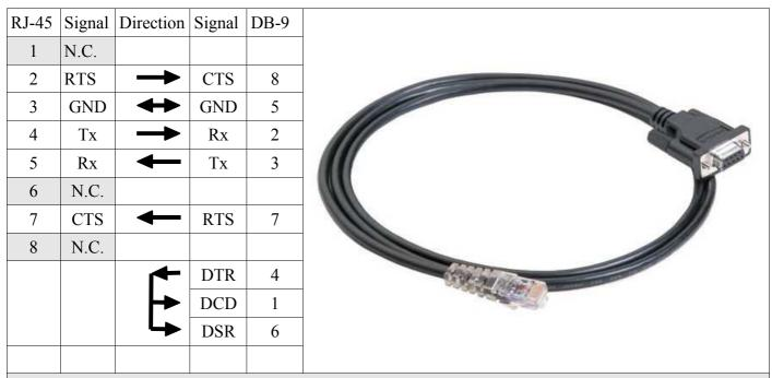
These pins are not connected on the RJ-45 Connector. They are reserved for DTR, DSR and DCD functions!
