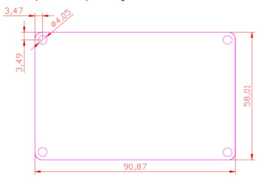
Figure 1: Schematic diagram of the size of the board
