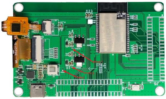
Figure 5: Schematic Diagram of Power Supply Test Point on Development Board
