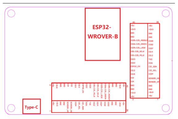
Figure 4: WT32-SC01 Interface Definition Diagram
