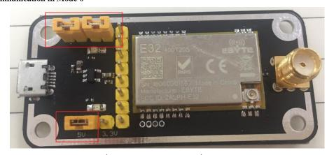
As shown above ,connect to jumpers( 5V power supply ,mode 0 ) ,both EXX-XXXTBL-01 are configured this way , open serial port , for data TX and RX , and AUX indicator is blinking.
