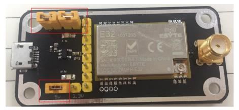
As shown in the figure, plug in the jumper (select 5V power supply, mode 0), both E22-900TBL-01 are configured as the same, open the corresponding serial port, you can send and receive data, and you can observe that the AUX light of the backplane flashes.
