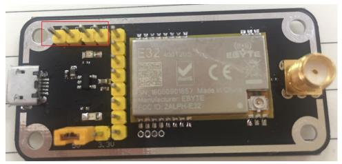
As shown in the figure, plug in the jumper (select 5V power supply, mode 3). For details, please refer to the corresponding serial port module manual.
