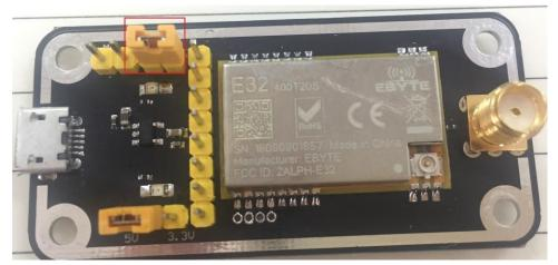
As shown in the figure, plug in the jumper (select 5V power supply, mode 1). For details, please refer to the corresponding serial port module manual.
