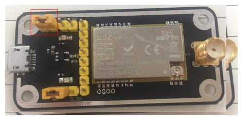
As shown in the figure, plug in the jumper (select 5V power supply, mode 2). For details, please refer to the corresponding serial port module manual.
